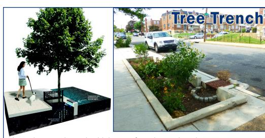
An underground trench with layers of sand, gravel, and stormwater storage. Soil, plants, and trees get planted and their roots can pull water from the storage beneath them. Good for high traffic areas and capturing stormwater with limited green space.
