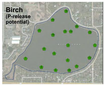
Lake Soil Survey: A total of 20 samples were collected on March 11, 2008 from depths ranging from 4 to 5 feet. Location of sample sites is shown in Figure A1. Samples in shallow water were collected using a modified soil auger, 5.2 inches in diameter. Soils were sampled to a sediment depth of 6 inches. The lake soil from the sampler was transferred to 1-gallon zip-lock bags and sent to the University of Minnesota Soil Testing and Research Analytical Laboratory.
