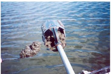
Figure A2. Soil auger used to collect lake sediments in water depths to 5 feet.
