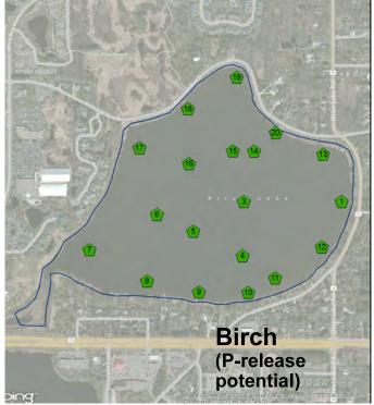
Figure 3. Sediment sample locations are shown with a circle. The color indicates the potential for phosphorus release from the sediments to occur at that site. Key: green = low potential.
