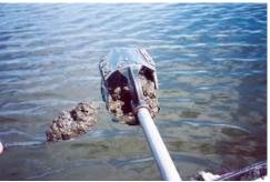
Figure 1. Soil auger used to collect lake sediments.
