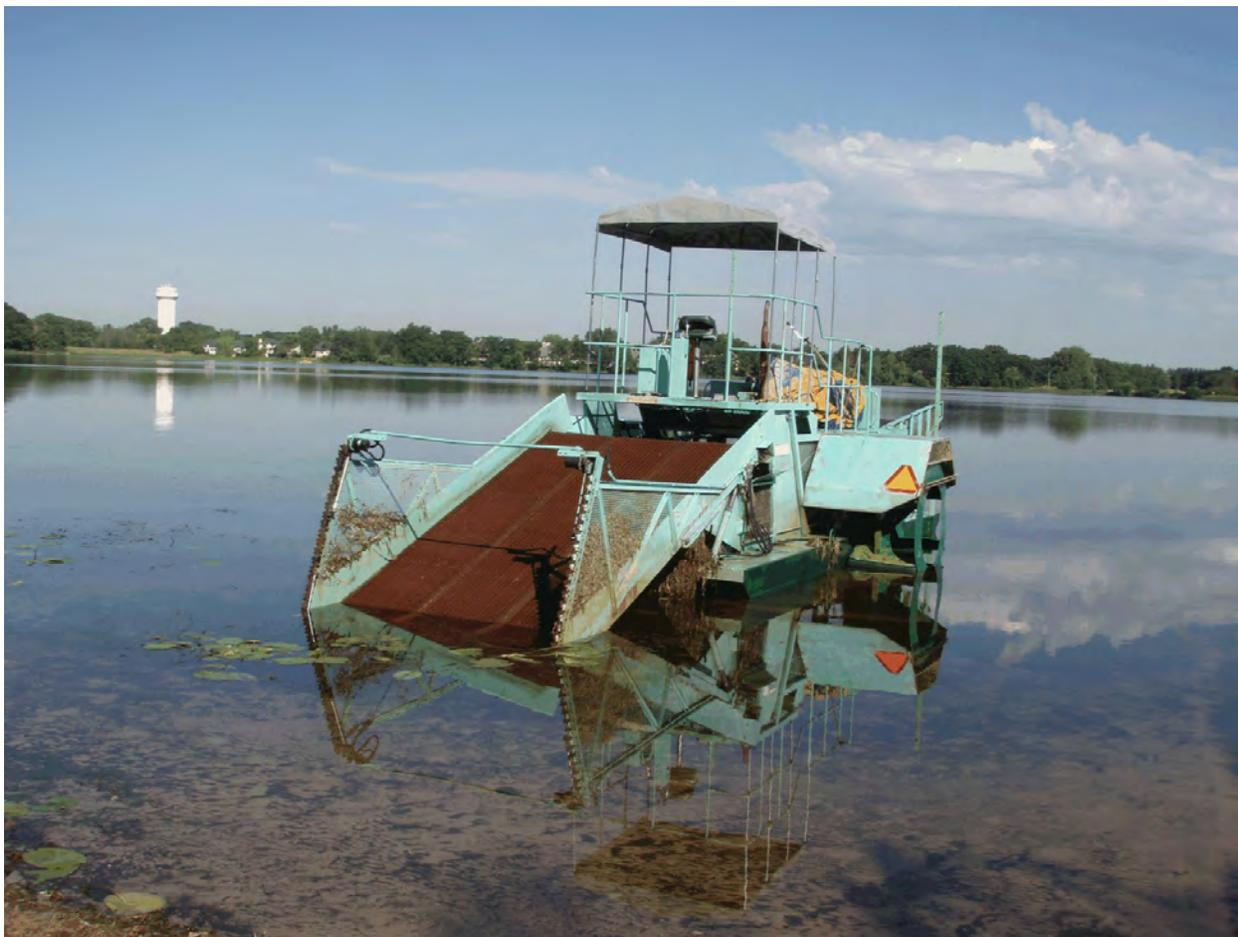
**Figure 12. A mechanical harvester used in Birch Lake is a good aquatic plant management option for heavy growth of pondweeds.**
