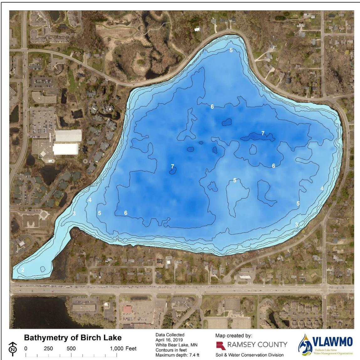
Figure 3. Depth of Birch Lake with 1-ft contours
