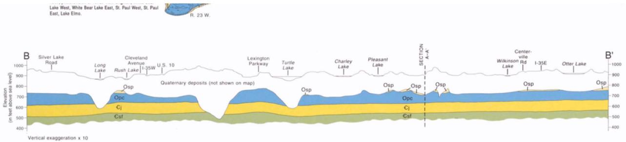
Figure A-8 Geologic cross-section of Pleasant Lake. Pleasant Lake is shown just to the left of the SECTION A-A dotted line. The white layer (Quaternary Deposits) is glacial till. The blue layer (Opc) is the Prairie Du Chein Group is a confined aquifer and the main contributing aquifer to Ramsey County. Notice that Pleasant Lake lies entirely in the glacial till layer and does not intersect with the Prairie Du Chein Aquifer (Meyer 1992).
