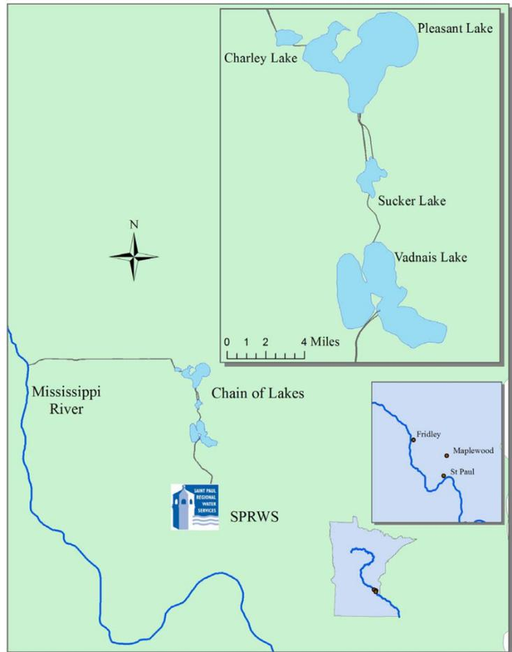
Figure 2.1.2 Map depicts the path of water transportation managed by SPRWS. The path begins at the Fridley pumping station and ends at the McCarrons treatment plant south of Vadnais Lake. (Map taken from project overview document)
