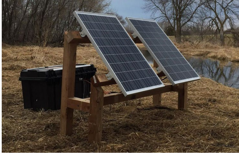
Figure 2. A solar array and work box for a PIT system. The data logger is located inside of the workbox and the antenna is placed in the water.
