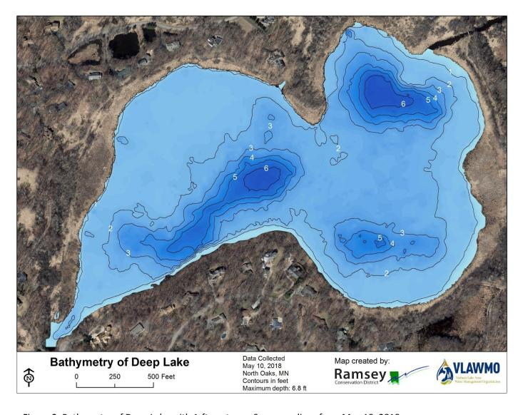
Figure 2. Bathymetry of Deep Lake with 1-ft contours. Sonar readings from May 10, 2018
