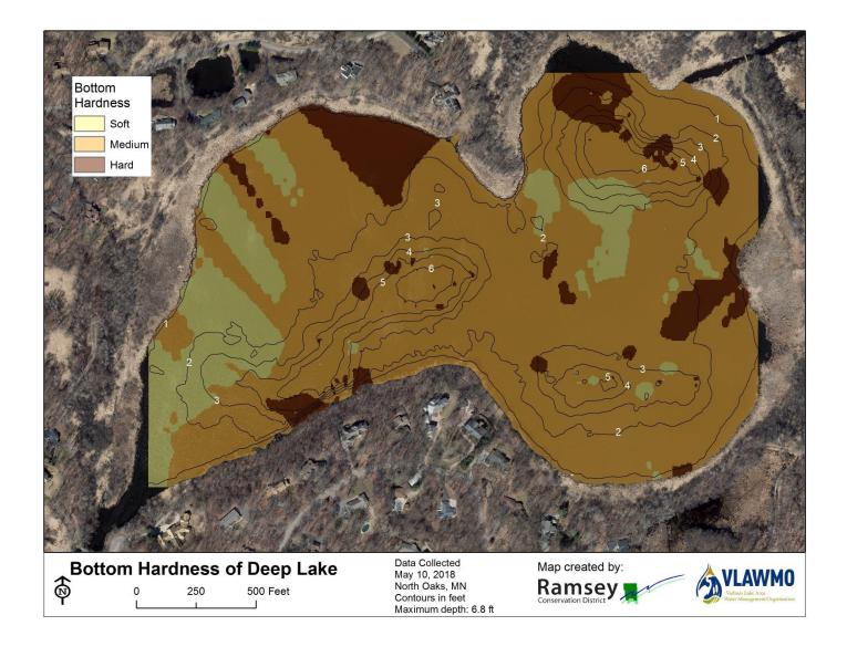
Figure 3. Bottom Hardness of Deep Lake with 1-ft contours
