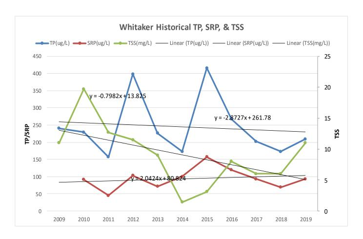
Whitaker Pond is above state standards for TP. State standard is 130 ug/l. State standard for TSS is 14mg/l. Since the forebay was installed in 2011 TSS has dropped, indicating the forebay is functioning as designed.
