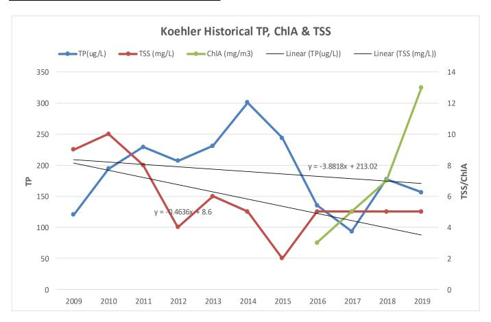
• State standard is 130 ug/l. State standard for TSS is 14mg/l. Stream bank restoration was done in 2011 and have noticed improvement in TSS levels over the years since restoration
