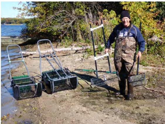
Use of small-scale controls that pick-up and remove zebra mussel clumps from the lake bottom could be considered. Modified clam rakes are an example of a small-scale zebra mussel removal tool that would be appropriate for a swimming beach or a boat landing area.
