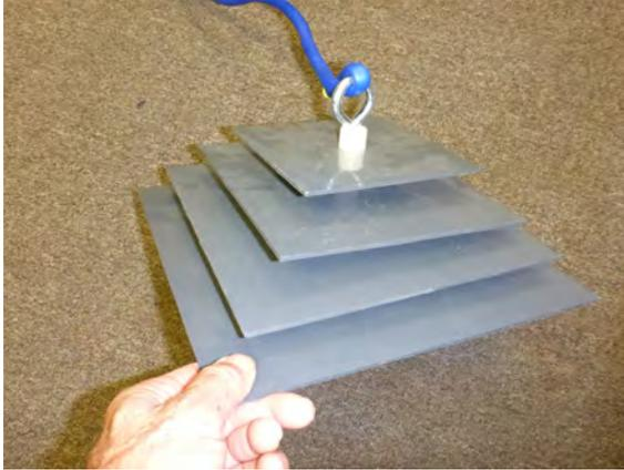
Figure 15. A zebra mussel plate sampler can be made from pvc materials. Ceramic tiles also make for good monitoring surfaces as well as pvc pipes.
