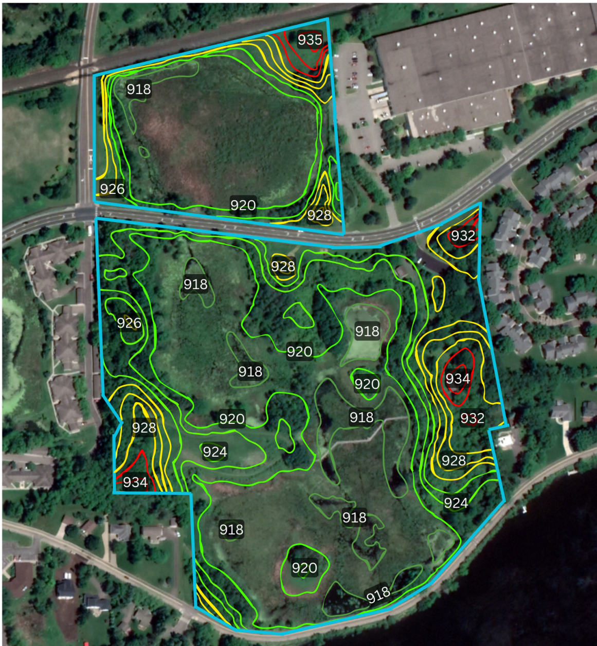
Appendix A, Figure 7 Elevation Levels
