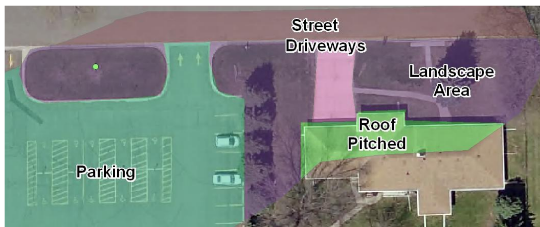
Figure 1. An example a neighborhoodsheds and the source areas that are entered into WinSLAMM (RCD, 2013, p. 7)
