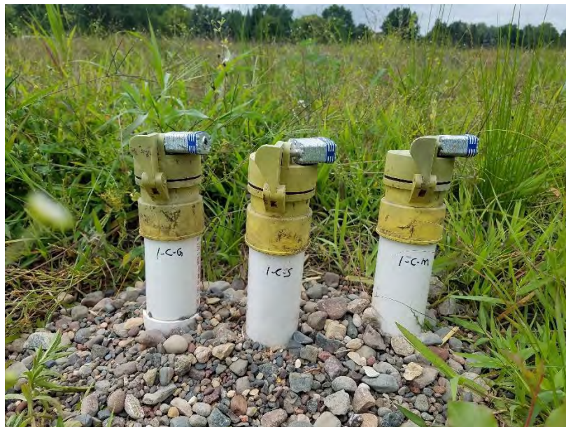
Figure 2-4: Photograph of Three Sampling Ports of a Monitoring Array Used to Collect Treated Water from Gravel (G), Sand (S), and Sorption Media (M) Layers in VFB Cell 1
