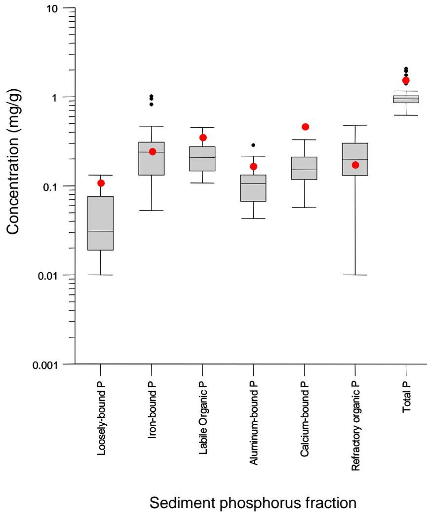
Figure 3. Box and whisker plots comparing various sediment phosphorus (P) fractions measured for sediment collected in the eastern basin of Goose Lake, MN, with statistical ranges for other lakes in Minnesota. Loosely-bound, iron-bound, and labile organic P are biologically-labile (i.e., subject to recycling) and aluminum-bound, calcium-bound, and refractory organic P are more inert to transformation (i.e., subject to burial). Please note the logarithmic scale.
