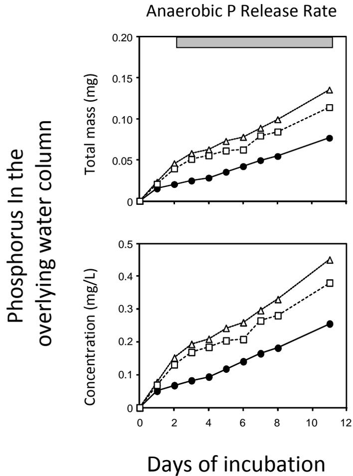
*Figure 1. Changes in soluble reactive phosphorus mass (upper panel) and concentration (lower panel) in the overlying water column under anaerobic conditions versus time for sediment cores collected in the eastern basin of Goose Lake. Gray horizontal bar denotes the time period used for rate estimation.*
