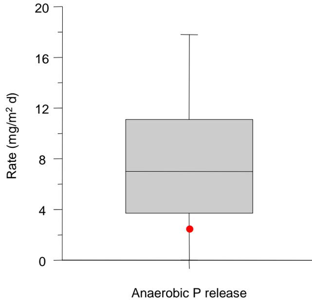
*Figure 2. Box and whisker plot comparing the anaerobic phosphorus (P) release rate measured for the eastern basin of Goose Lake (red circle) with statistical ranges for other lakes in Minnesota.*
