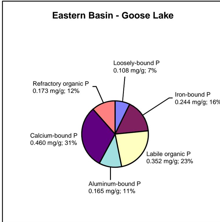
*Figure 4. Composition of biologically-labile phosphorus (P) in the upper 10-cm surface sediment layer of the eastern basin of Goose Lake. Loosely-bound, iron-bound, and labile organic P are biologically reactive (i.e., subject to recycling). Values next to each label represent concentration ( $\text{mg}\cdot\text{g}^{-1}$ ) and percent of the biologically-labile P concentration, respectively.*
