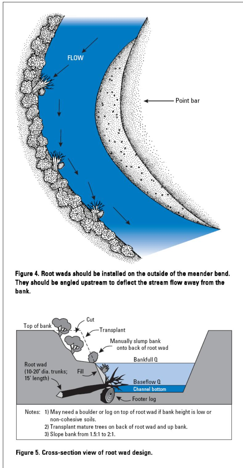
**Figure 4.** Root wads should be installed on the outside of the meander bend. They should be angled upstream to deflect the stream flow away from the bank.
