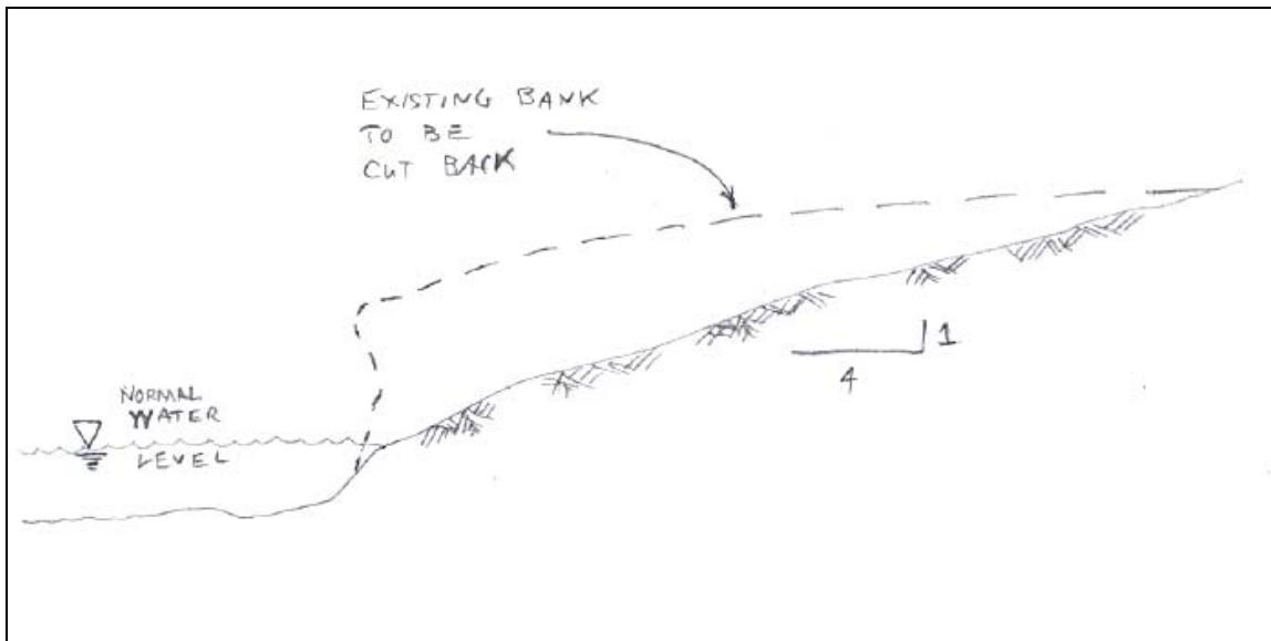
**Figure 35. Generalized bank re-shaping.**
