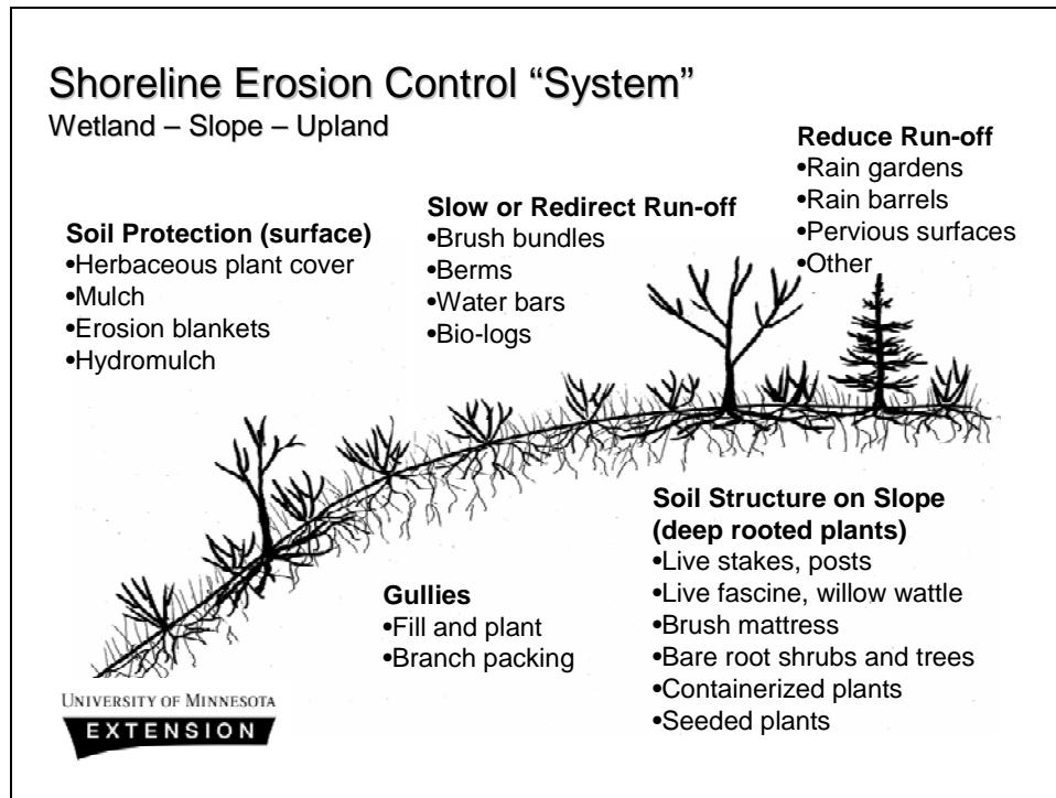
**Figure 56. Bioengineering methods to be used in combination for erosion control of slope and upland.** (Minnesota Shoreland Management Resource Guide, <http://www.shorelandmanagement.org/index.html> All rights reserved.)
