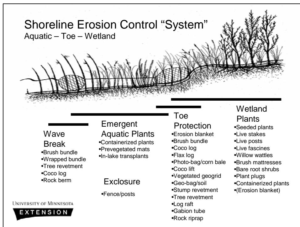
**Figure 55. Bioengineering methods used in combination for shoreline stabilization.**
