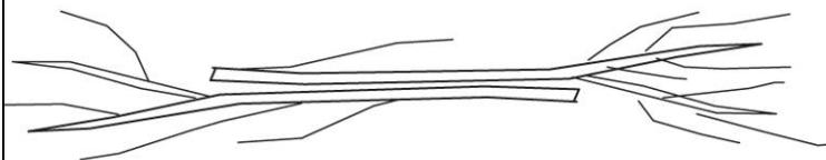
1. Assemble brush bundles by alternating butt ends with brush tops facing toward the outer edges. Before laying out first branch place a thick diameter rope ( $\frac{3}{8}''$  to  $\frac{1}{2}''$ ) underneath the staging area to help cinch the branches together for steps two and three below.
