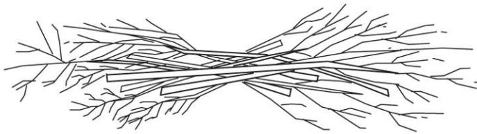
2. Keep stacking and assembling brush bundles until there is large enough bundle to cinch together. Use the cinch technique until the bundle is tight enough to add additional branches to the bundle. Cinch again as necessary.
