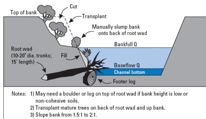
**Figure 5.** Cross-section view of root wad design.
