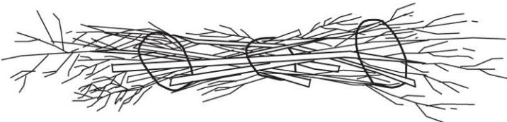
3. Use the thicker diameter ropes to cinch the bundle into a tight two foot by ten foot brush bundle. After tightening with rope use an organic twine or equivalent diameter rope to reduce inter twig gaps and create a tightly formed wave break bundle 2-3 foot in diameter by 10-12 feet in length.
