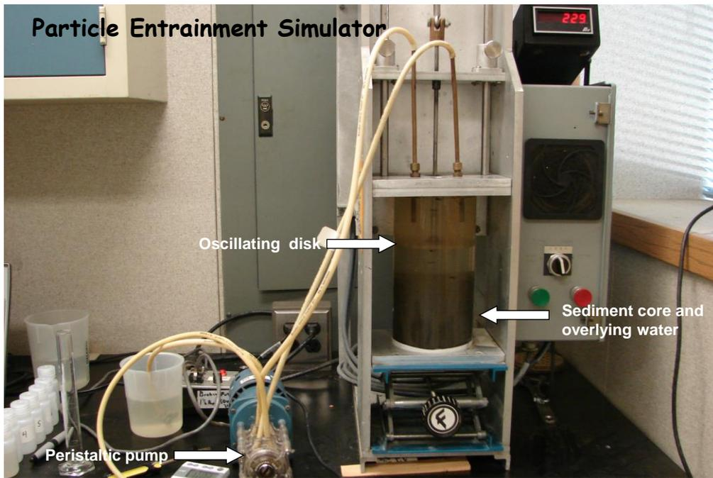
*Figure 2. Simulation of sediment resuspension using a particle entrainment simulator (PES).*
