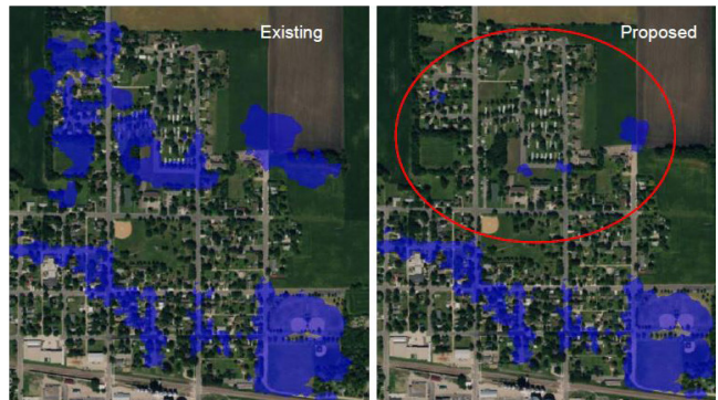
1D/2D XPSWMM model results, showing existing and proposed conditions for one alternative
