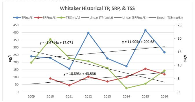
• Whitaker Pond on average for the last 8 years is above state standards for TP. State standard is 130 ug/l. State standard for TSS is 14mg/l. Since the forebay was installed in 2011 TSS has dropped, indicating the forebay is functioning as designed.
