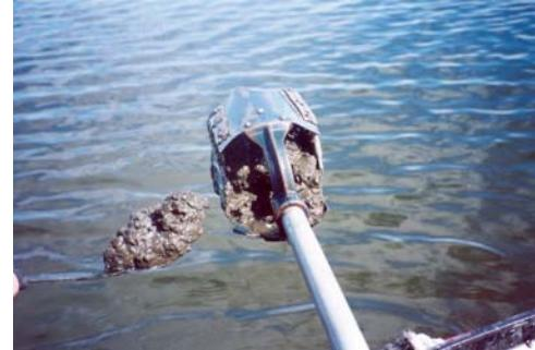
**Figure 1. Soil auger used to collect lake sediments.**
