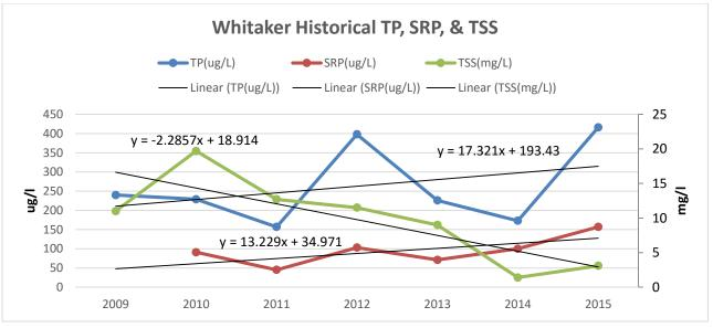
• Whitaker Pond on average for the last 7 years is above state standards for TP. State standard is 130 ug/l. State standard for TSS is 14mg/l. Since the forebay was installed in 2011 TSS has dropped, indicating the forebay is functioning as designed.
