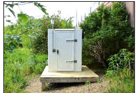
Barr has installed several creek monitoring stations, including this station on Purgatory Creek.
