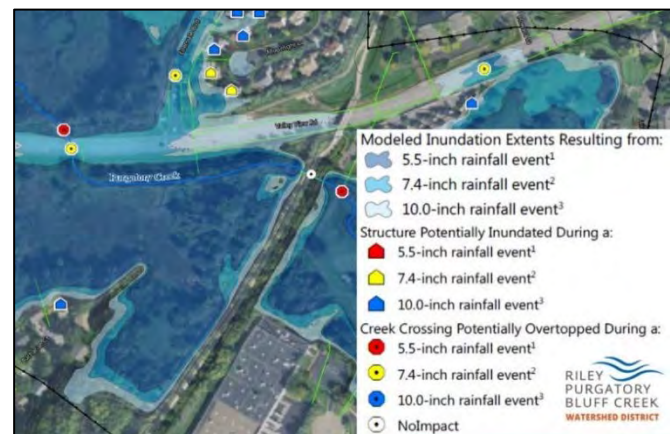
Flood inundation areas and vulnerable structures/ roadways were mapped based on a range of rainfall depths.
