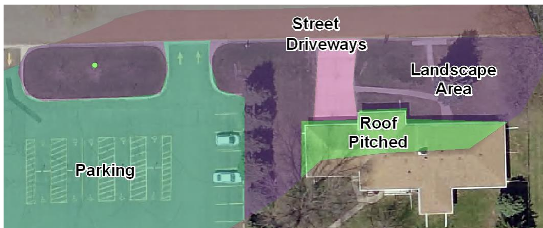
Figure 6. An example neighborshed and the source areas that are entered into WinSLAMM
